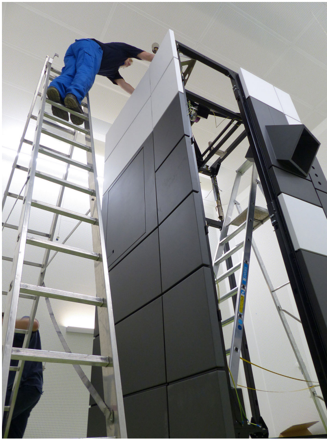
The four-meter-high housing of the SALVE microscope is mounted
