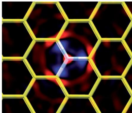
**Figure 2** | DFT results for the changes in electron density due to bonding. The blue (red) colour shows a lower (higher) electron density than in the case in which the independent atomic model is used<sup>1</sup>.
