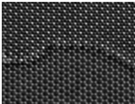
**Figure 1** | HRTEM image of single and bilayer graphene with atomic resolution.
