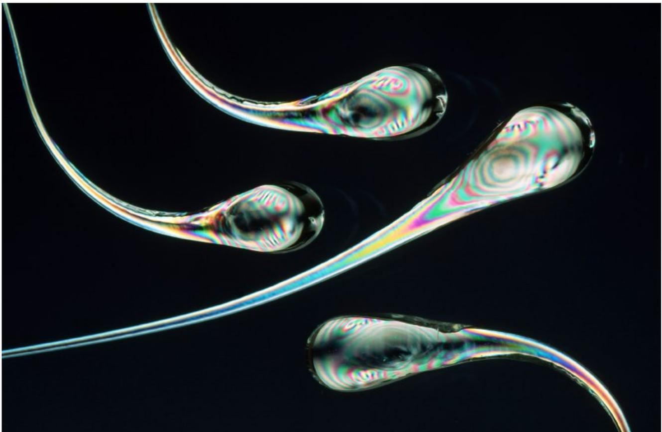
Glass suddenly cooled in water: The „Prince Rupert Drop“ resists even hammer blows, but breaks immediately if his tail is damaged - due to internal stresses.
